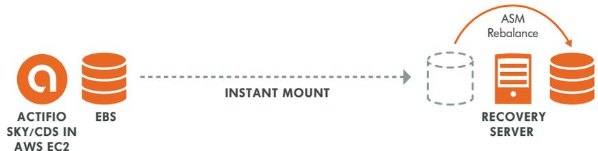
Actifio automates this by integrating with ASM rebalance where the changed blocks, post-recovery, are transparently replicated back to production storage in the background.
