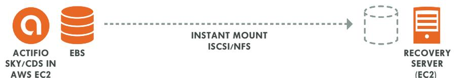
Actifio Sky mounts the point-in-time backup image (which is in native Oracle format and not a traditional RMAN backup) to an AWS EC2 instance over iSCSI/ NFS and recovers the database in minutes. Based on the specified point in time, it automatically replays any archive logs that are needed.
